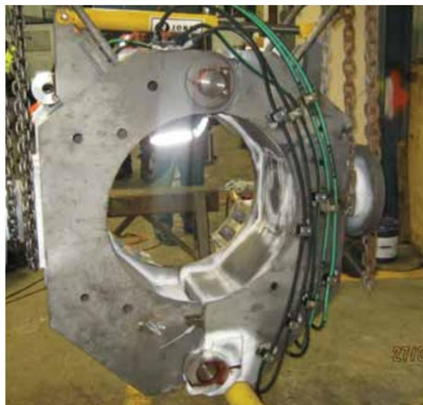
The finished Hydraulic Clamp before testing
