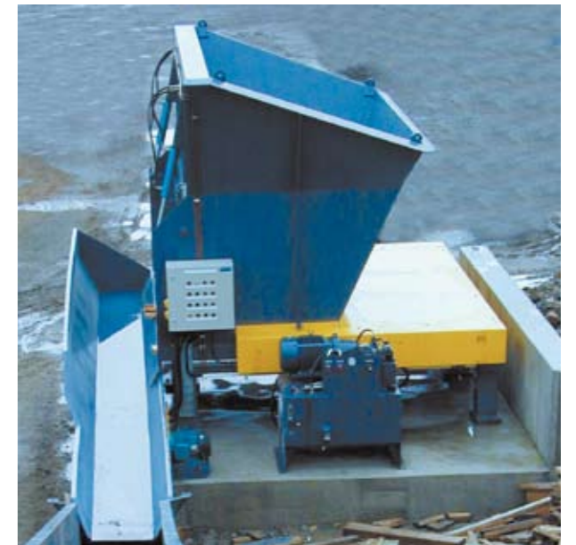
Loader Reception Bunker
