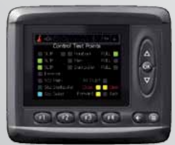
Visual Test Points Fault Identified
