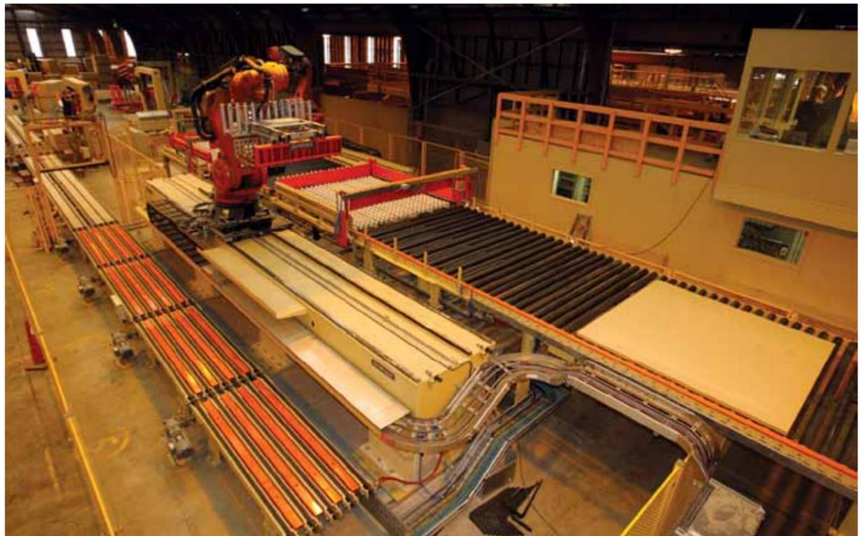
Anthon Robots load packs into the Fromm strapping stations.
