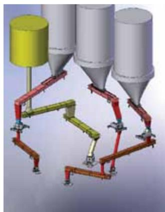
Layout drawing of the BEL supplied equipment for one boiler.
