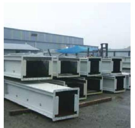
Completed CCMW en masse conveyor sections ready for dispatch.
