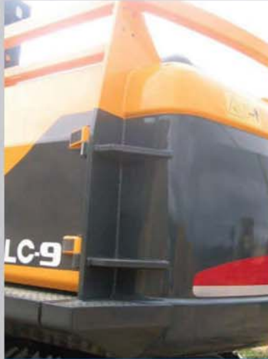
Rear kicker plate to protect doors and provide secure hinge and rail mounting
