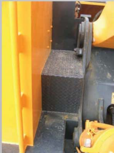
Access steps in toolbox to allow easy access to engine
