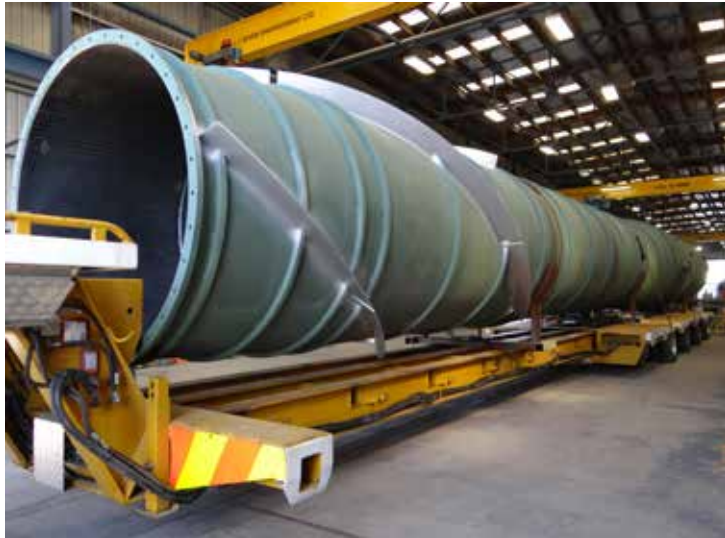
Boiler Stack ready for transport
