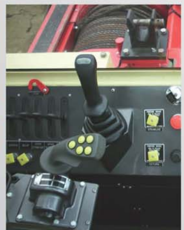
Single Lever Joysticks for Winch Control
