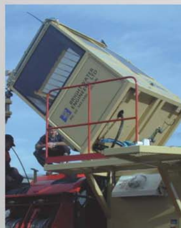
Hydraulic Tilting Cab
