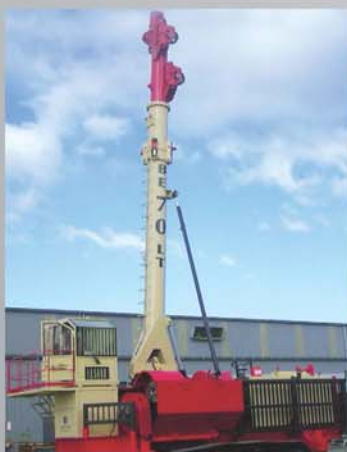
70ft (21m) Telescoping Tower
